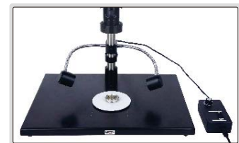
illumination direction and brightness are adjustable
