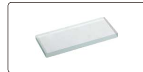
50mm reading scale (check magnification accuracy)
