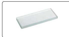
50mm reading scale (check magnification accuracy)
