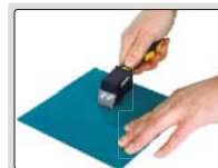
step 1: make grid cutting on surface
